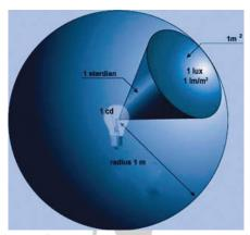
If the source and its radiation angle is small, the brightness will appear to be intense even if its emission is small. Therefore the apparent brightness of this source when looking directly into it should be differentiated from its luminous emission, that should be described by candela per square meter.
