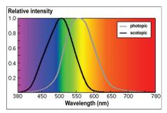
Using this curve that is possible to make a relation between experienced human sensation of light with measurable physical concept of energy. The sensors used for light intensity measurement meet with the standards describing curves for photopic and scotopic vision.
